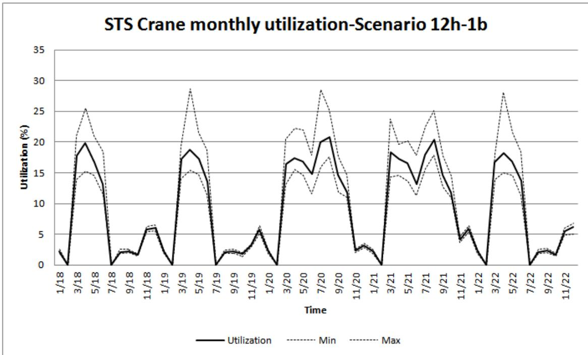
Figure A. 7. Monthly STS Crane Utilization for Scenario 1
