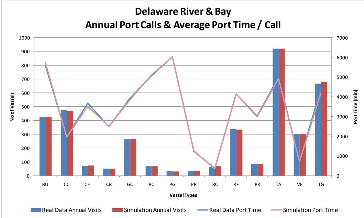
Figure 2 Validation results on vessel port calls and port times
