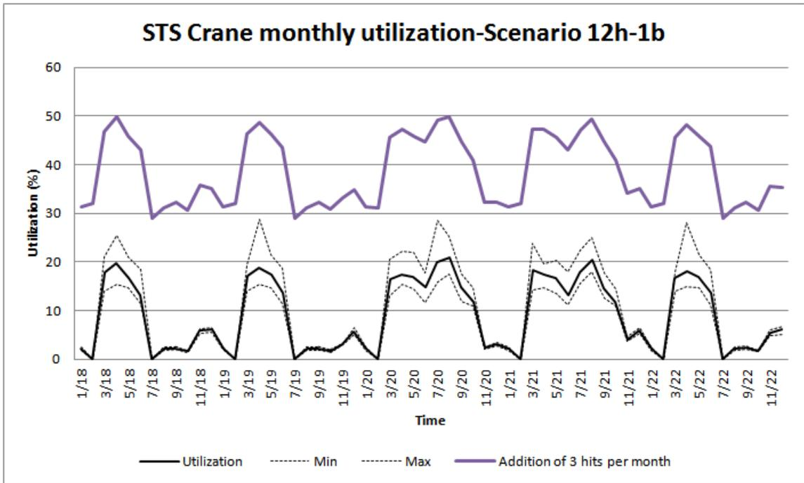
Figure 9. STS Crane monthly utilization including 3 extra shipments for Scenario 1
