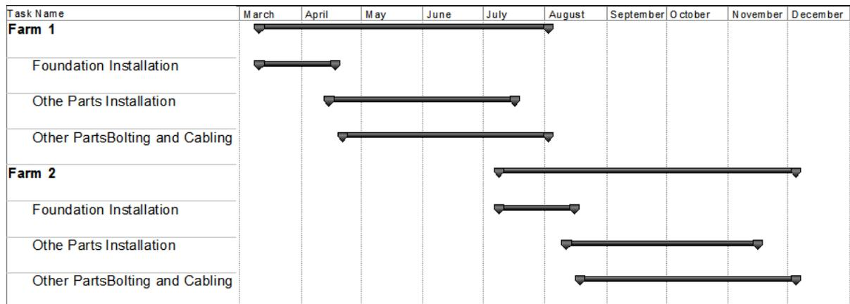
Figure 5. An example project plan for installation of 60 turbines in 9 months
