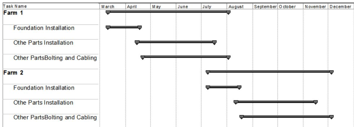
Figure 5. An example project plan for installation of 60 turbines in 9 months
