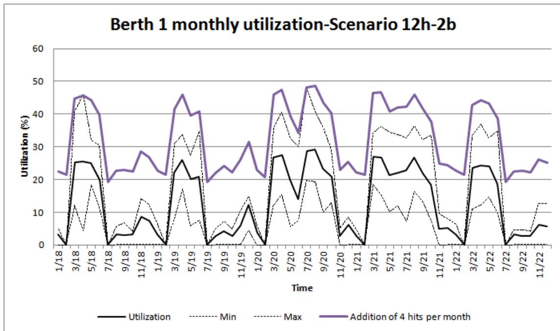
Figure 10. Berth 1 monthly utilization including 5 extra shipments for Scenario 3
