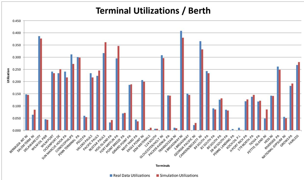
Figure 3 Validation results on terminal utilizations
