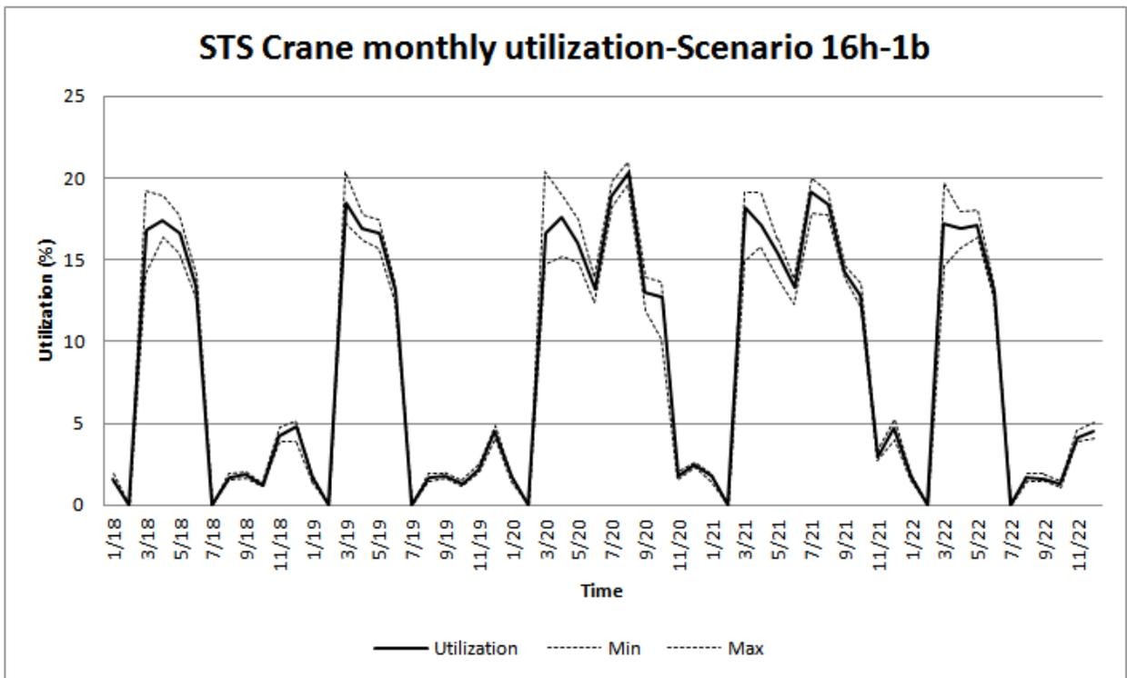
Figure A. 23. Monthly STS Crane Utilization for Scenario 2
