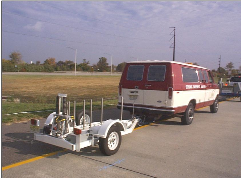
**Figure 26: Seismic Pavement Analyzer (SPA)**
