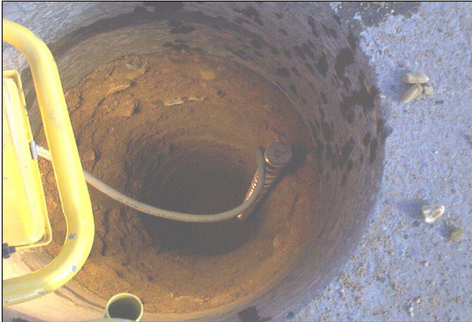
**Figure 22: Resistivity Probe**
