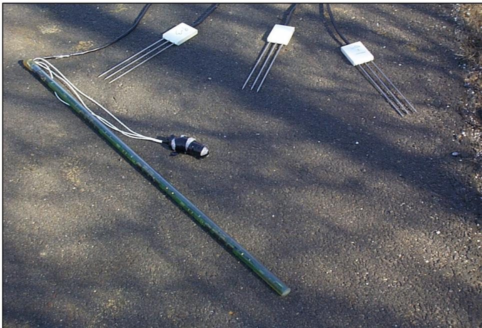
**Figure 21: TDR and Temperature Probes**
