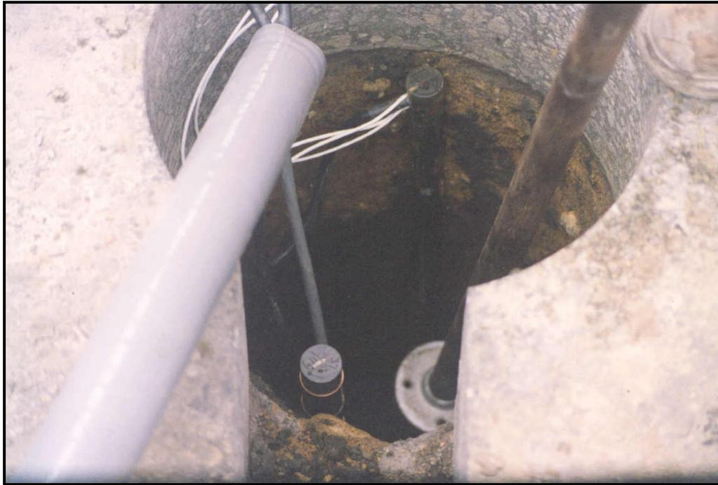
**Figure E.3: Installing MRC and Thermistor Probes**
