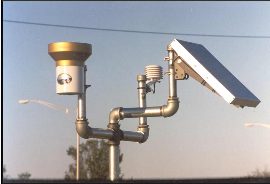
**Figure 20: Tipping Bucket, Solar Panel, and Air Temperature Probe**
