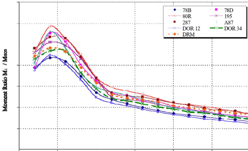
Figure 98. Seventy-five-year predicted negative moment ratio by span for New Jersey WIM sites
