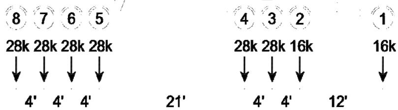
Figure 68. Permit vehicle from NJDOT *Bridge Design Manual* (NJDOT 2002)
