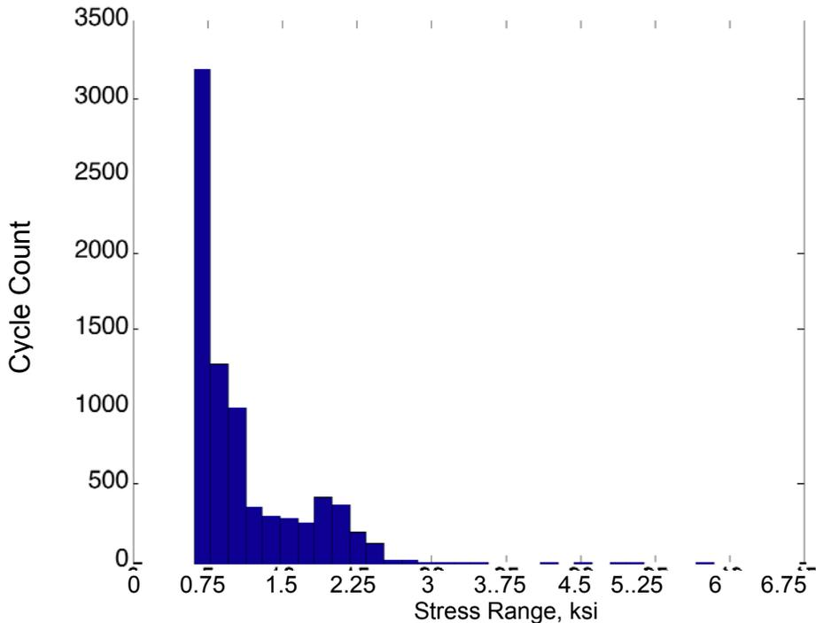
Figure 105. Results of semi-continuum simulation neglecting truck superposition.
