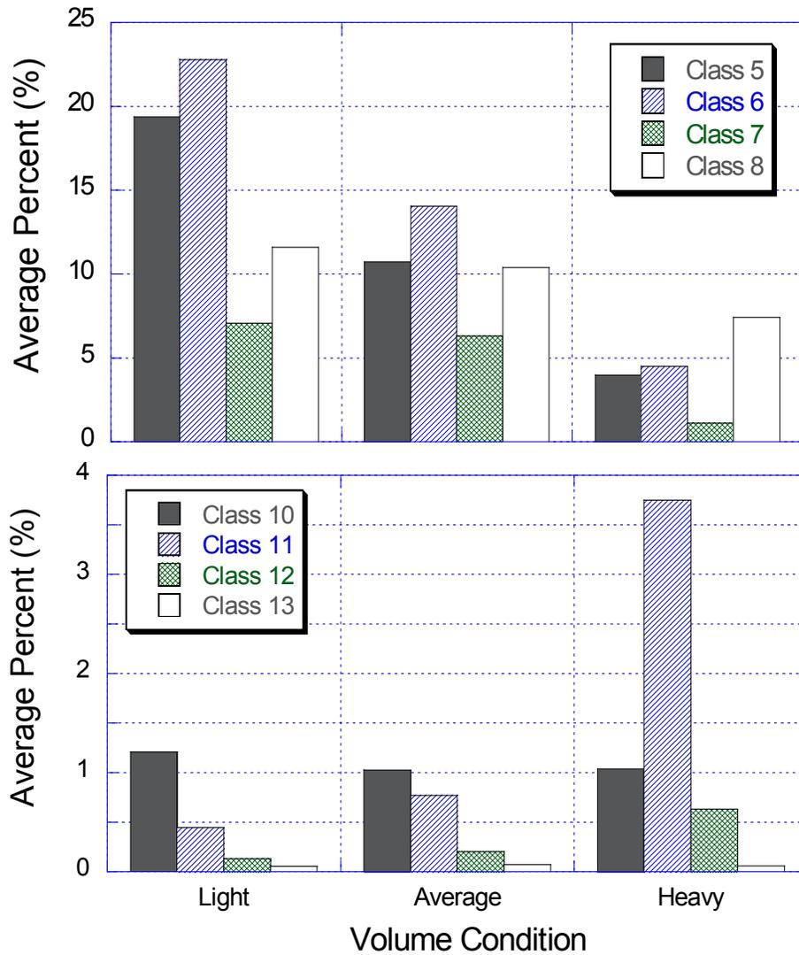
Figure 60. Vehicle type by site volume condition (33 sites, June 2003)
