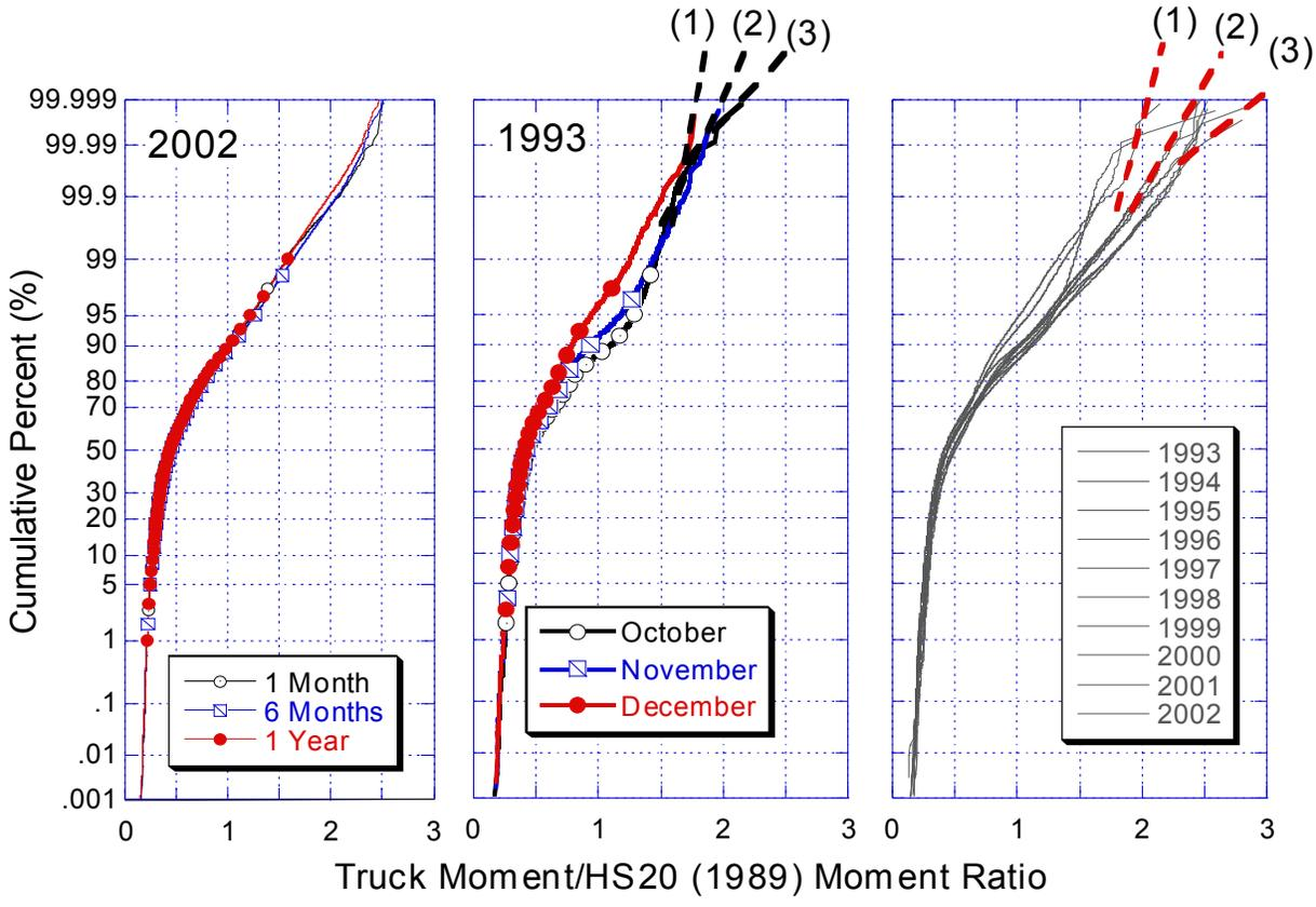
Figure 67. Bridge live-load effects and extrapolation based on various time periods (Site 195)
