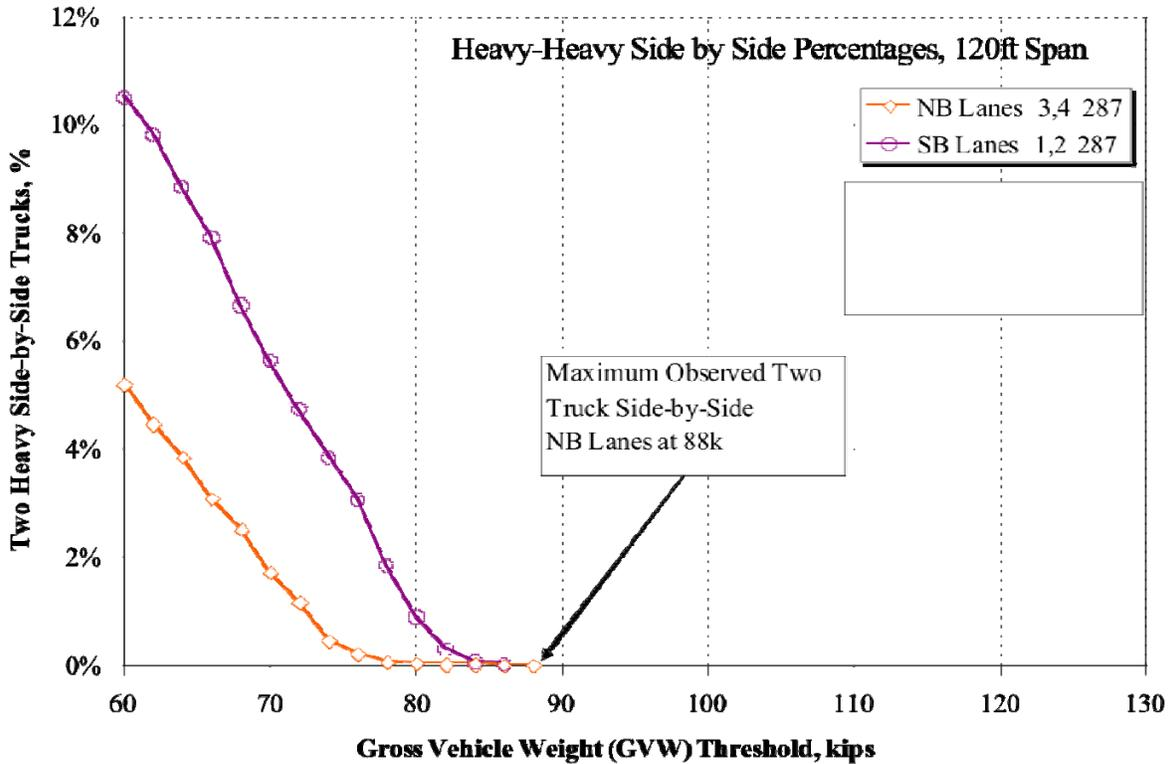
Figure 84. New Jersey WIM Site 287: variation of side-by-side event statistics for two heavy trucks using different “heavy” weight thresholds for a span of 120 ft
