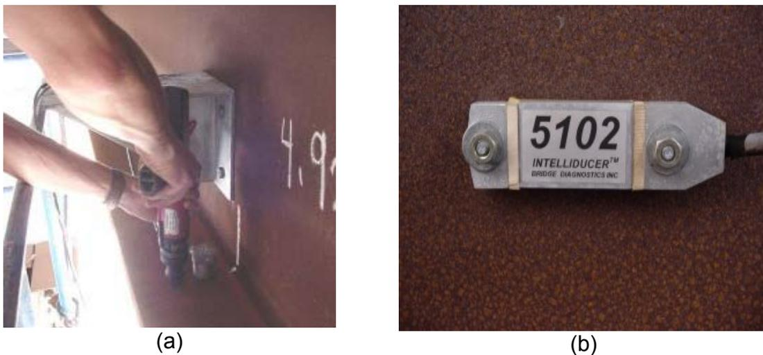
Figure 6. (a) Gauge installation and (b) mounted strain transducer
