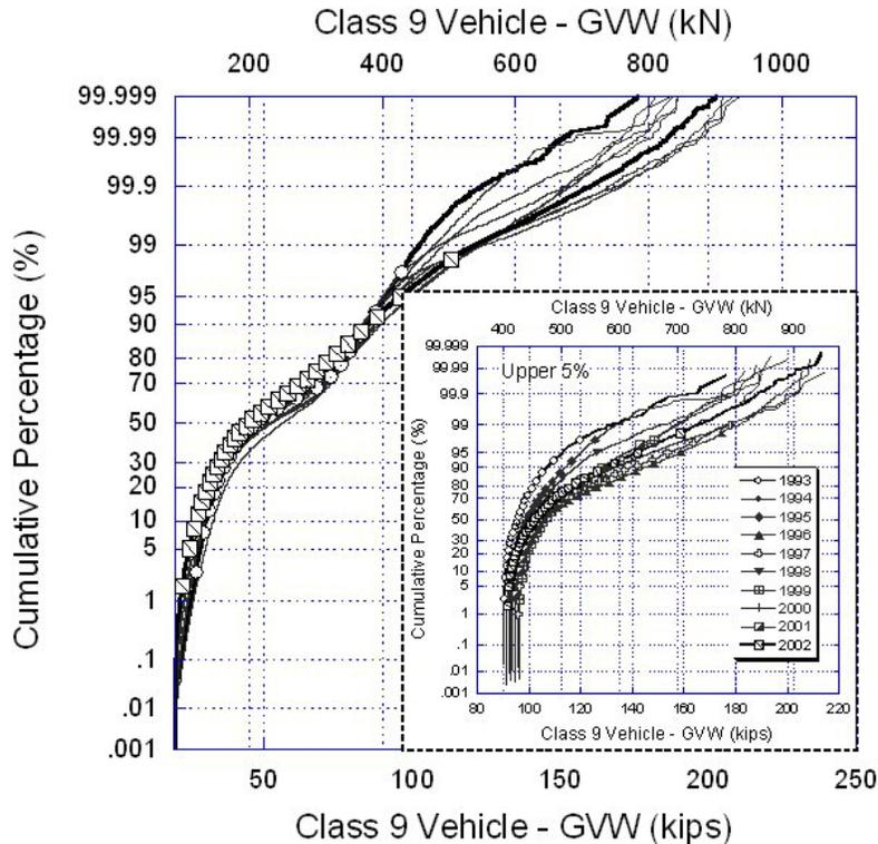
Figure 66. Total truck weight for Class 9 vehicles (Site 195)
