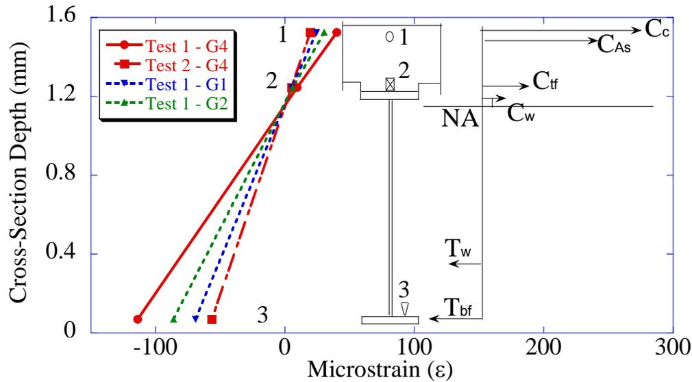
Figure 51. Neutral axis location on Span 1
