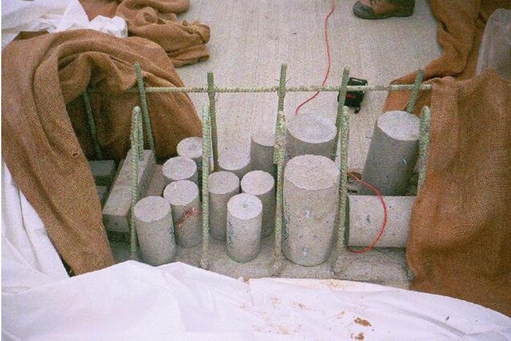
Figure 14. Field matched-cured specimen
