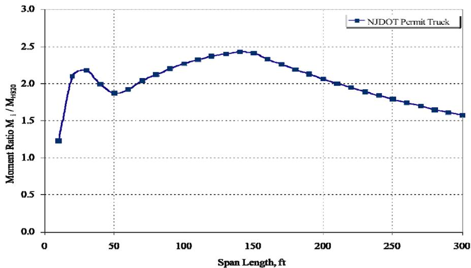
Figure 69. Simple moment envelope for NJDOT permit truck
