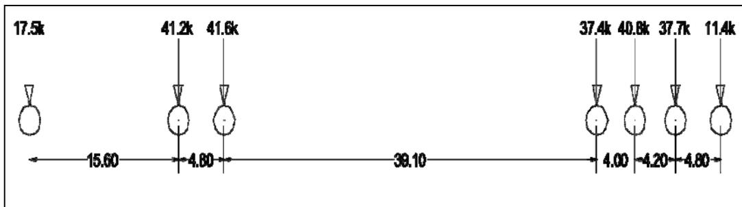
Figure 102. Extreme heavy truck observed at Doremus Avenue Bridge on 5/11/04 (weights are in kips, spacing in feet)
