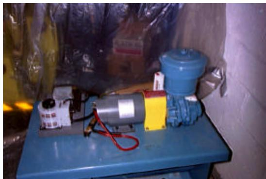
Figure 18 Fuel cell air compressor assembly.
