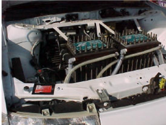
Figure 20 Two 7 kW (gross) fuel cell stacks installed in a vehicle.
