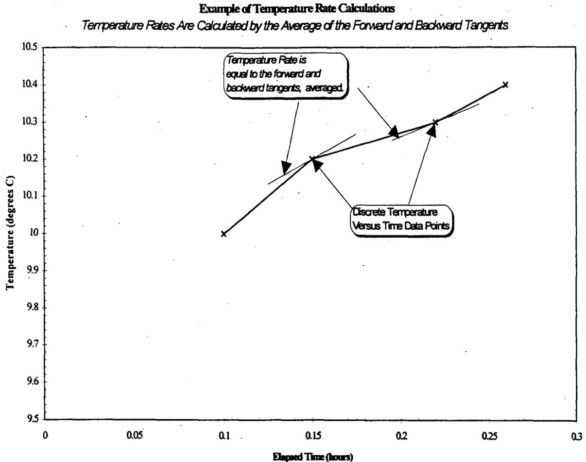
*Figure 2.4 Example of Temperature Rate Calculations From Typical Temperature-Time Plots*
