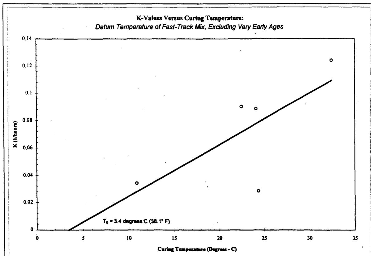
By excluding the very early age data points, the computed datum temperature reflects the datum at later ages, approaching infinity. This datum is only applicable after about 12 hours elapsed. With the K-values determined, the long-term datum temperature can be estimated. A best-fit line is made for the five K-values, previously computed. From the best-fit line, the datum temperature is 3.4° C (38.1° F)
