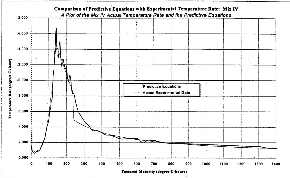
**Figure 2.12 Comparison of Predictive Equations with Experimental Temperature Rate: Mix IV**
