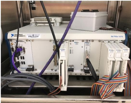
(b) Chassis with input modules and a controller
