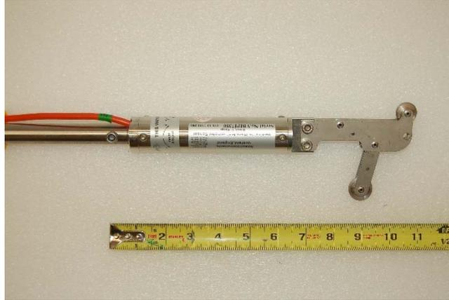
**Figure 3.2 In-place inclinometer (IPI) sensor**
