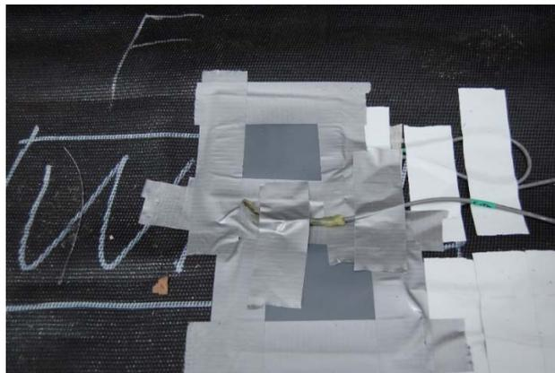
**Figure 3.12 Thermistor installation**
