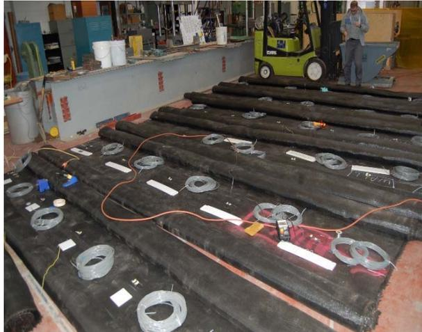
**Figure 3.9 Strain gauge wiring in the University of Delaware lab prior to site installation**
