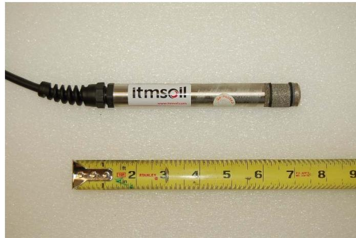
**Figure 3.4 Piezometer sensor**
