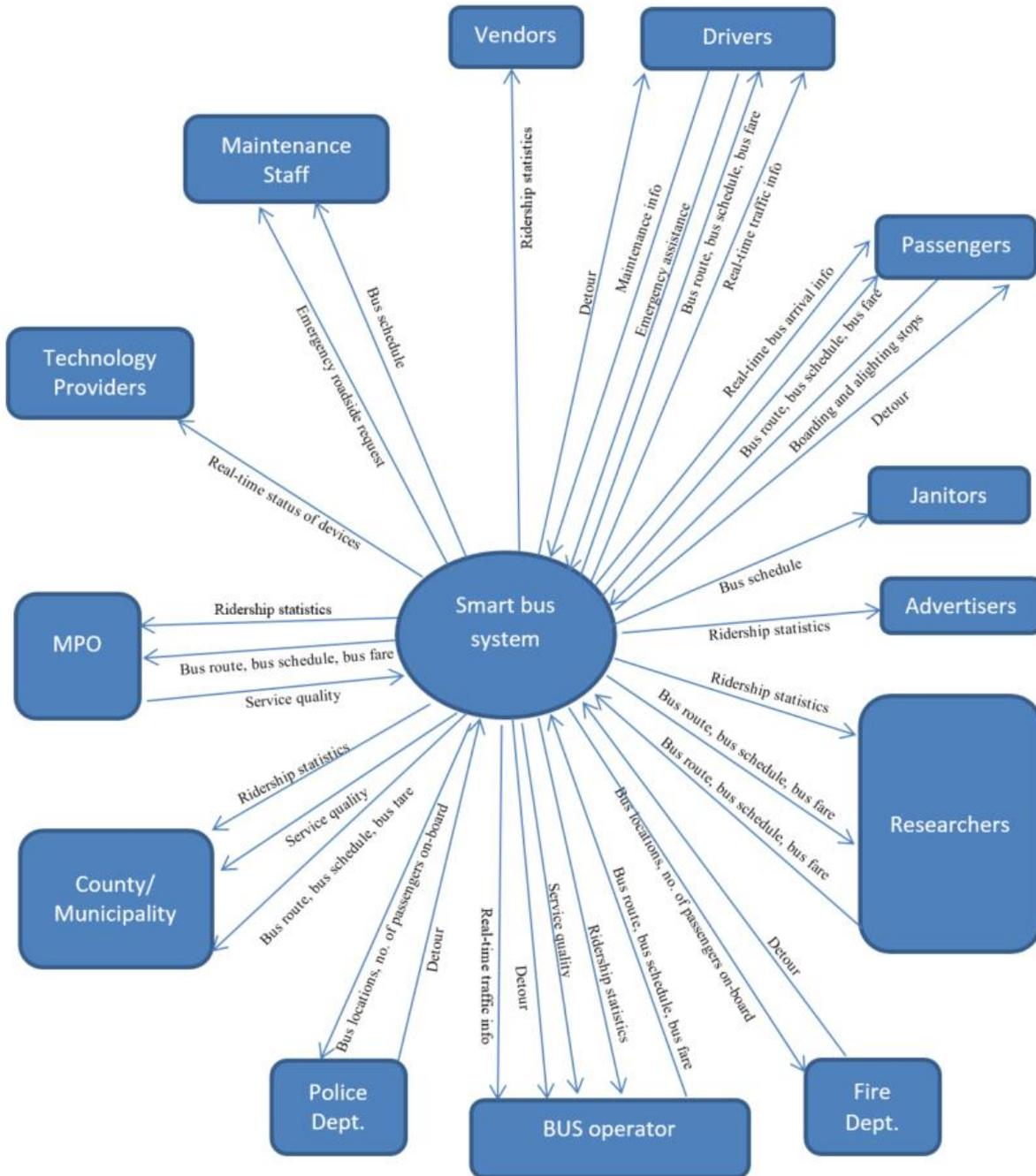
Figure 5.6 Level zero system diagram for smart bus systems
