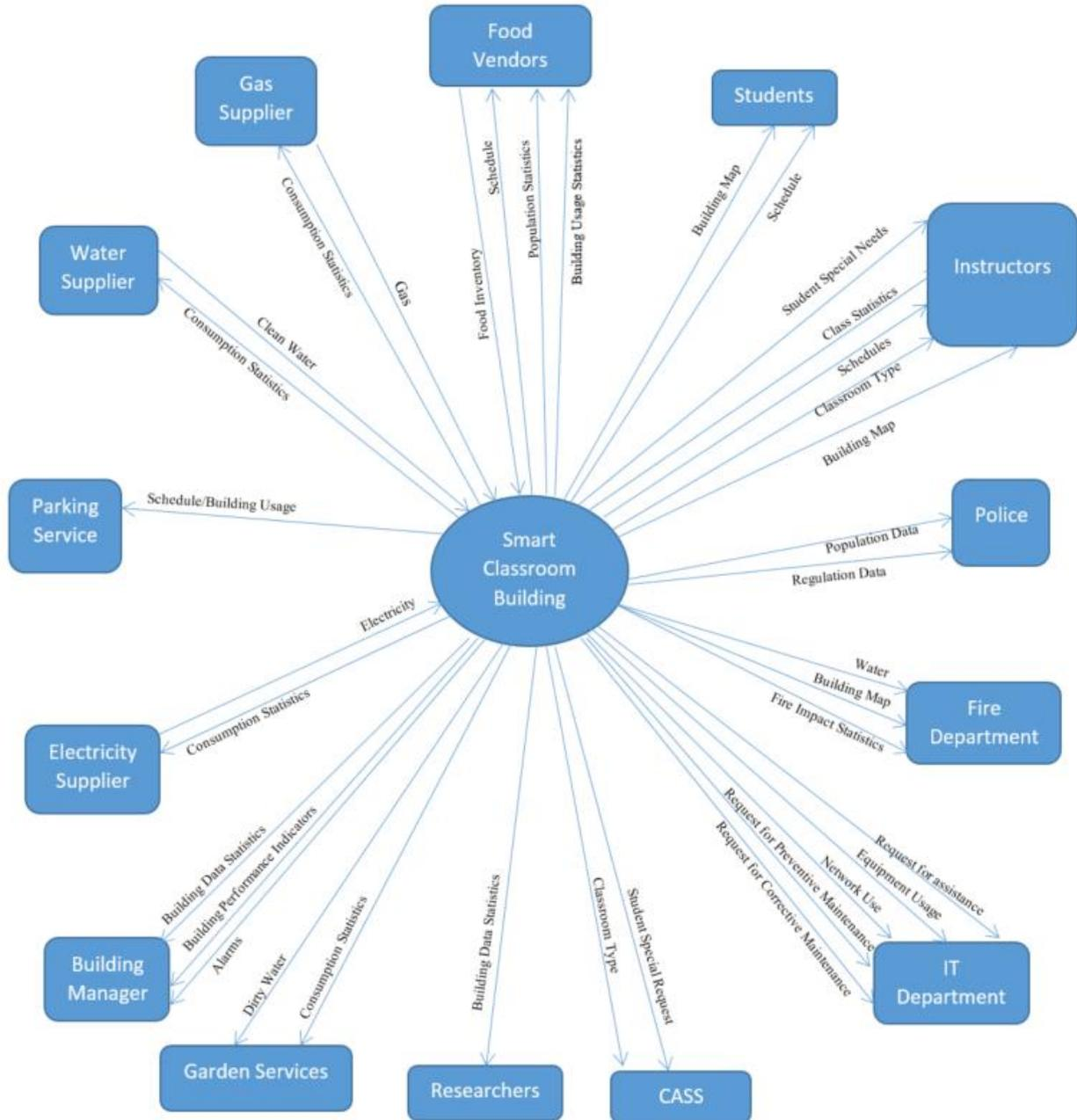
Figure 3.5 Level zero system diagram for smart classroom buildings
