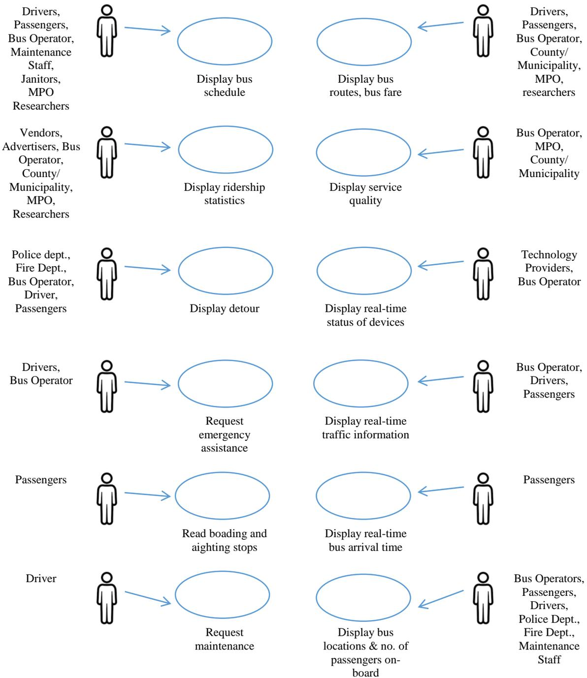
Figure 5.6 Use case diagrams for smart bus systems
