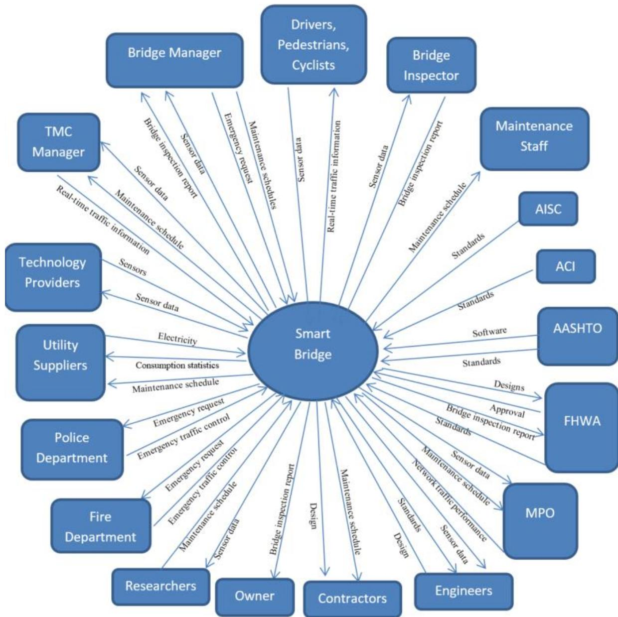
Figure 4.5 Level zero system diagram for smart bridges
