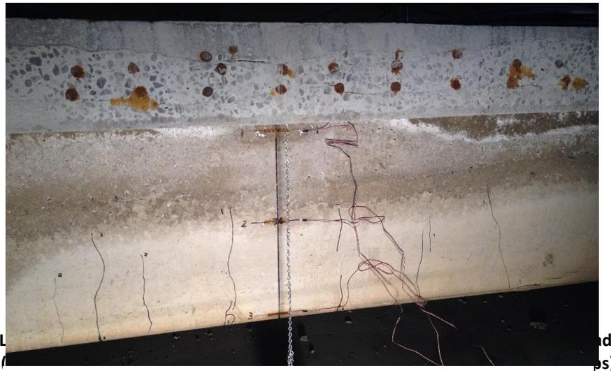
Figure 3.15 Strain gages and marked cracks on Girder #1
