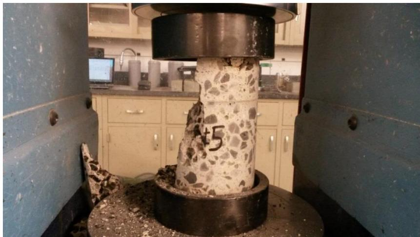
Figure 4.2 Concrete cylinder after failure
