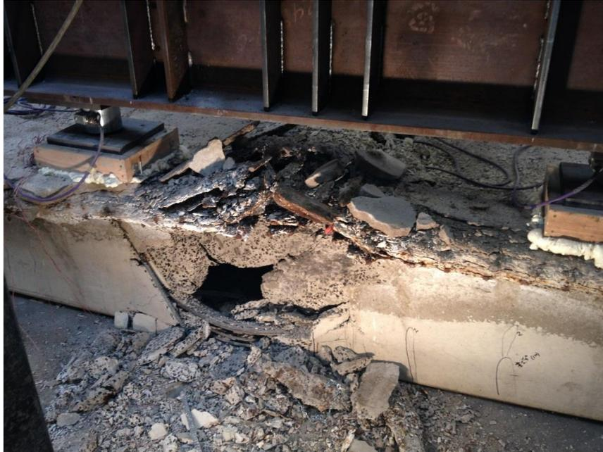
Figure 3.17 Girder #1 after flexural failure
