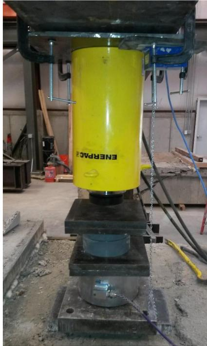
Figure 3.32 Typical punching shear test setup
