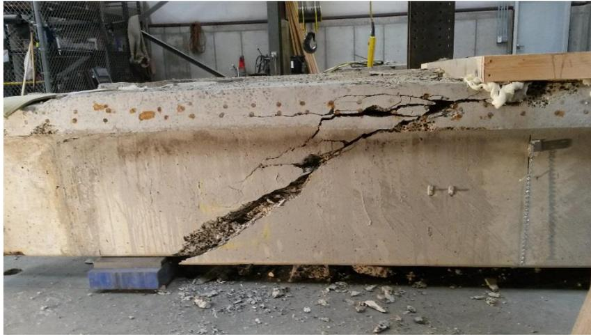
Figure 3.25  $3d_v$  shear failure of Girder #2
