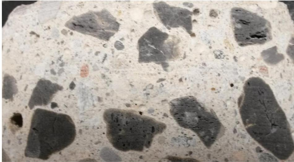
Figure 4.3 Concrete aggregate
