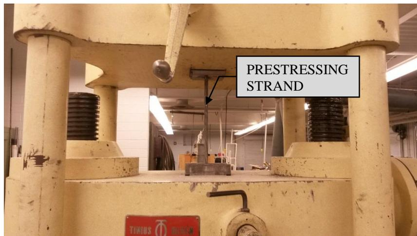
Figure 4.4 Prestressing strand test setup
