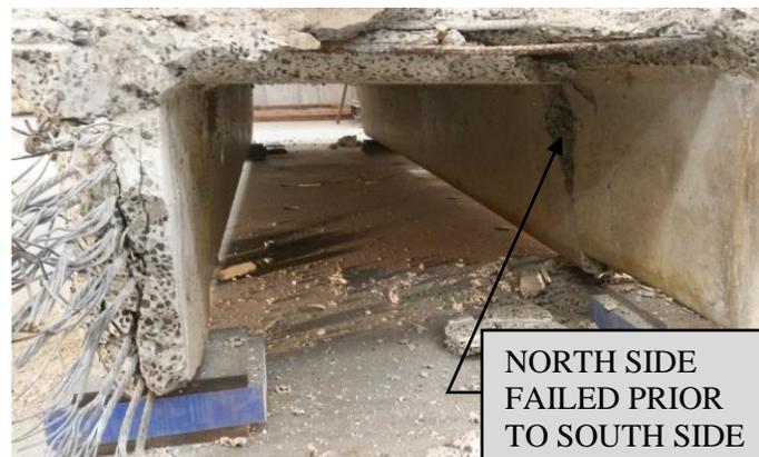
Figure 3.30 Girder #3  $2d_v$  failure
