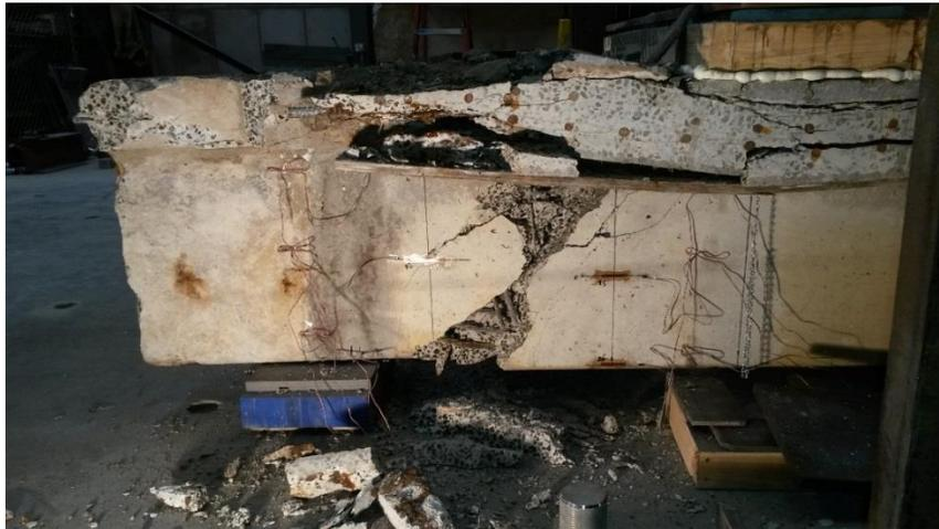
Figure 3.24  $2d_v$  shear failure of Girder #1
