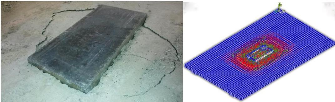
Figure 5.11 Punching shear 3D view
