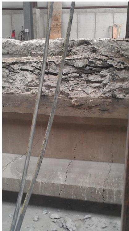
Figure 28 Cracks and crushes prior to failure
