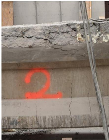
Figure 25 Cracks under the loading location prior to ultimate failure
