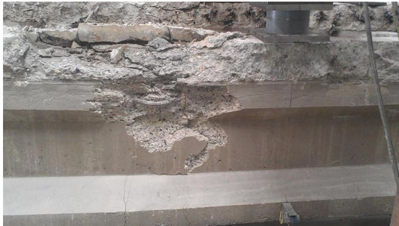
Figure 34 Compressive failure in G7-4d(a)
