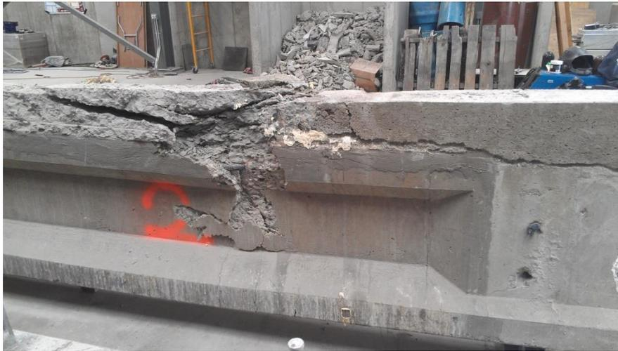
Figure 27 Compressive failure for G2-1d(a)
