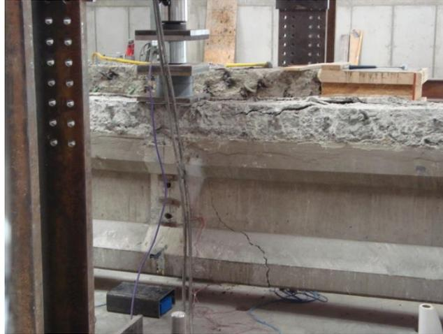
Figure 14 Cracking during midspan flexural test
