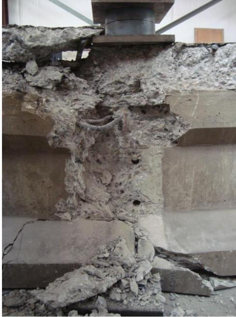
Figure 15 Ultimate failure for midspan flexural test
