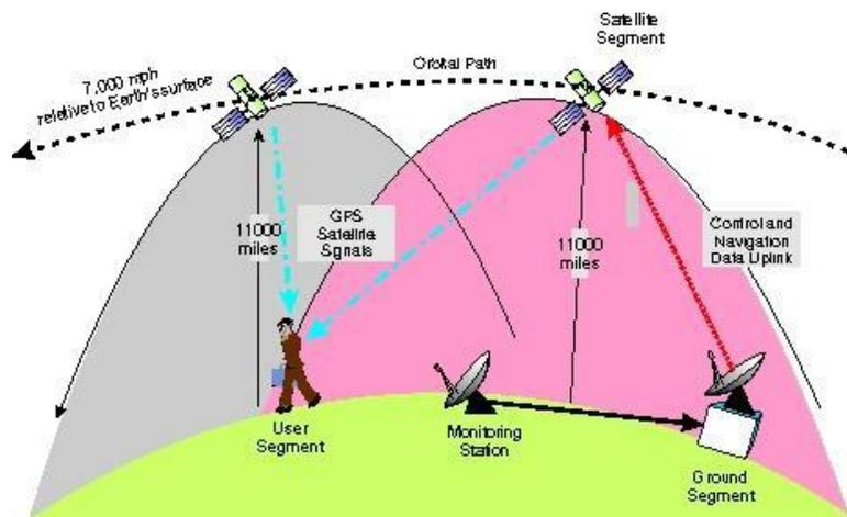
Figure 3 The Principle of GPS Positioning
