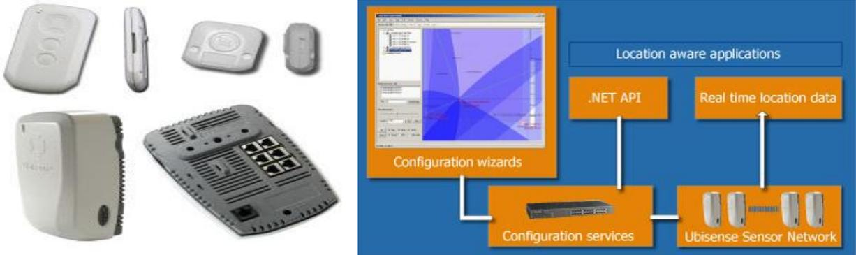
Figure 5 Typical Components in a UWB system (Ubisense 2013)
