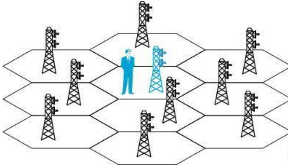
Figure 6 A Cellular-based RTLS System (Credit: [www.cisco.com](http://www.cisco.com))
