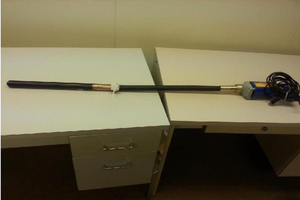
Figure 12 A Concrete Vibrator with an Attached UWB Tag
