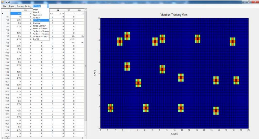
Figure 14 The Interface of the Vibration Effort Tracking System
