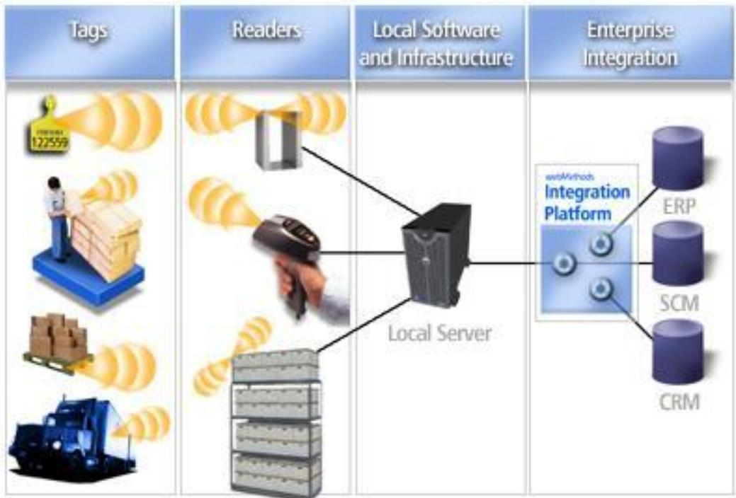
Figure 4 RFID System Components (Winthrop 2006)
