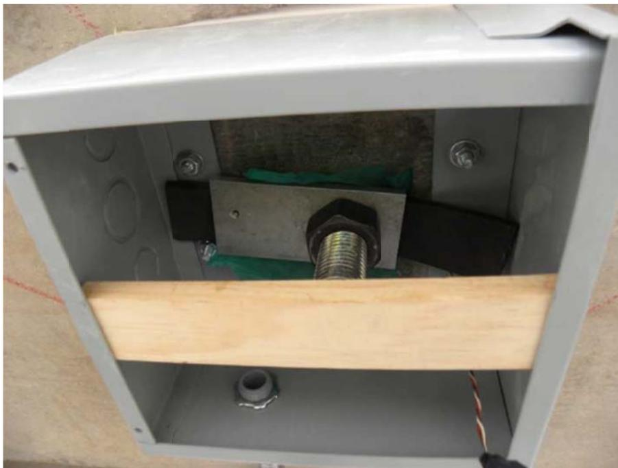
*Figure 4.5 View of installation method for hitec foil strain gauges*
