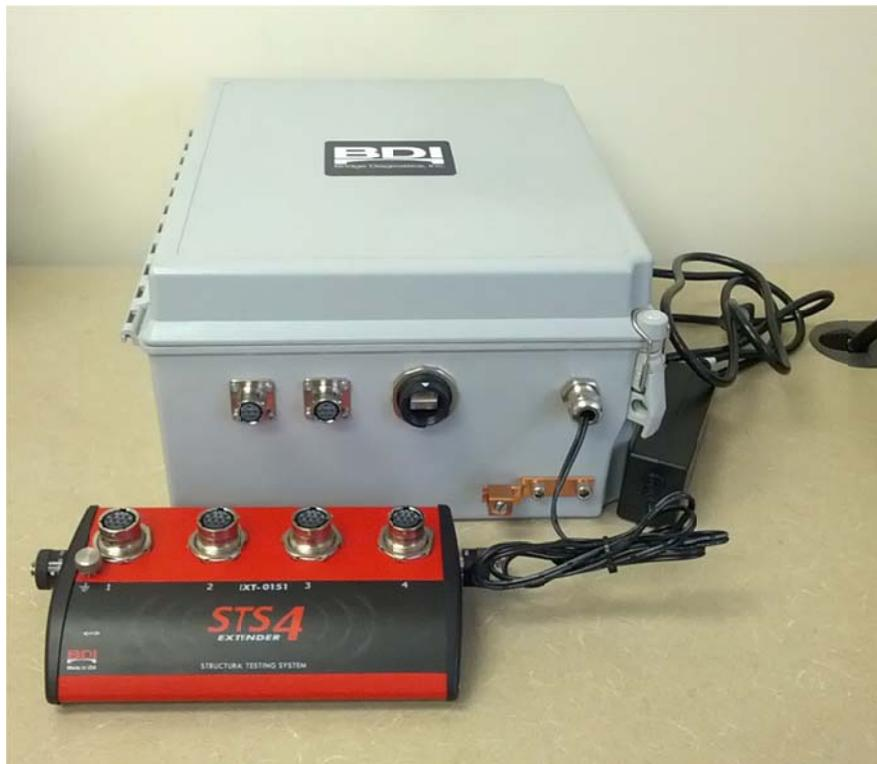
*Figure 10.20 The STS4 testing system*
