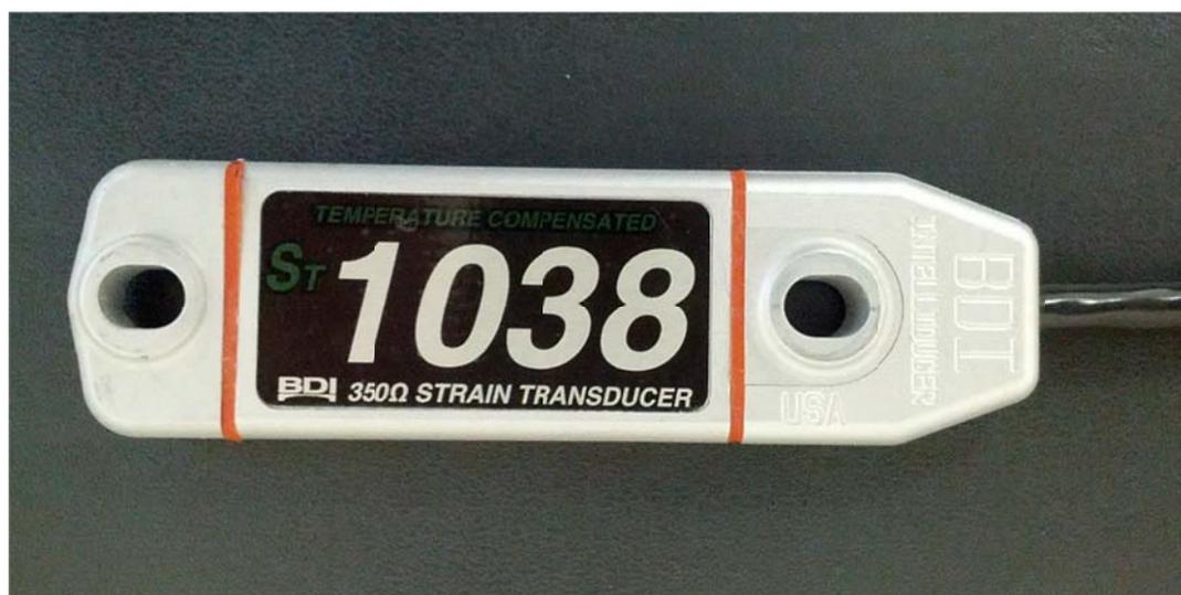
*Figure 10.7 BDI Strain Transducer*
