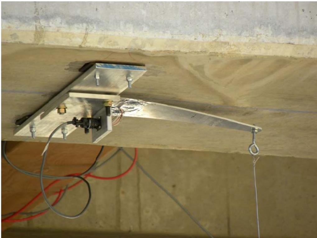
*Figure 6.2 Deflection instrument, "deflectometer"*
