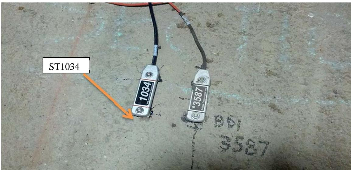
Figure 10.33 Set-up of strain gauge next to existing at Section F, this is the trigger gauge
