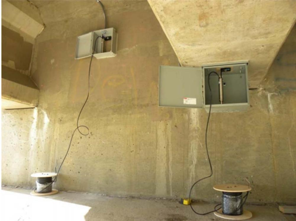
*Figure 3.4 Showing two tiltmeters installed one on girder and one on abutment*
