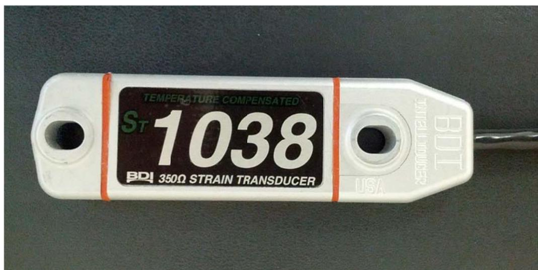
*Figure 10.7 BDI Strain Transducer*
