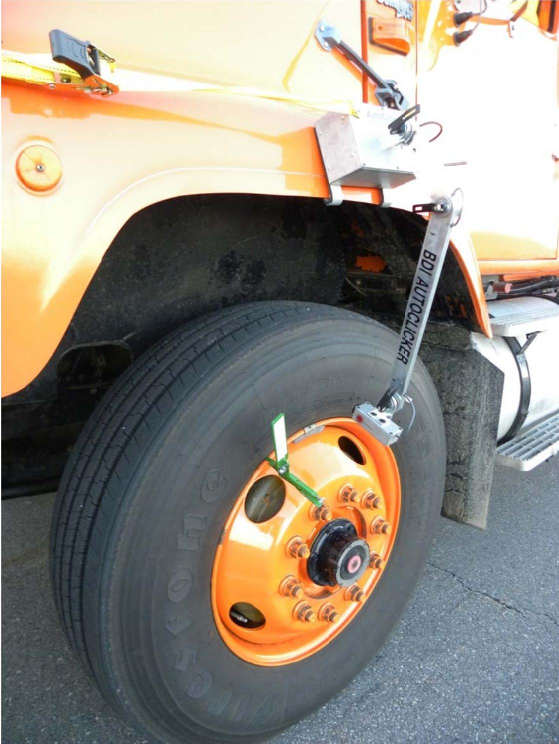
*Figure 6.16 Automated position tracking sensor, "Autoclicker," mounted on left front tire of Truck A*
