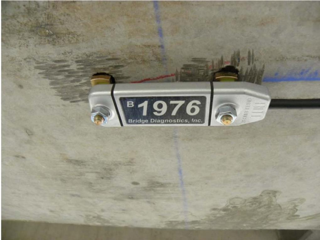
*Figure 6.1 Surface mounted strain gauge*
