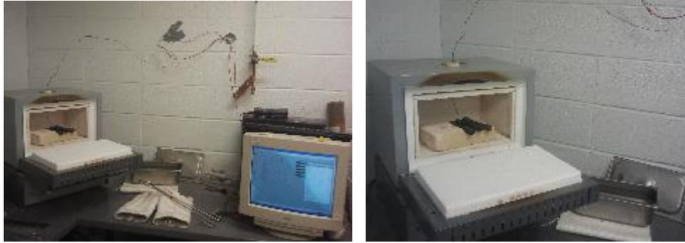
**Figure 9.** (a) Heating and cooling test setup. (b) Furnace with three standard round specimens placed inside. The companion specimen is on the far right (with the thermocouple sticking out from one side), while the two specimens that will be mechanically tested after they have been heated and cooled are to the left of the companion specimen.
