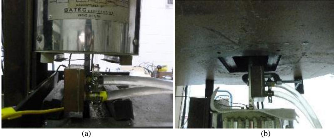
**Figure 13.** Close up images of the cooling plates attached to the (a) bottom and (b) top of the specimen as it left the furnace. The cooling plates were made of copper with cold water continuously running through them to remove heat from the specimen before it reached the clamps.
