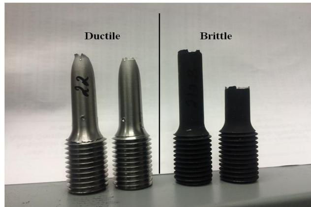
**Figure 23.** Ductile and brittle failure of Material 1 test specimens. Ductile failure is shown on the left for specimen 1A (unheated) compared to brittle failure observed on the right for specimen 1Cw-1500.
