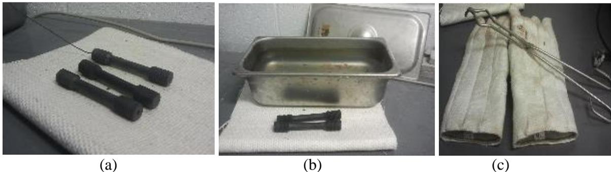
**Figure 10.** (a) Companion specimen (with thermocouple inserted) along with two mechanical test specimens cooling in air on top of a ceramic blanket; (b) two mechanical specimens after being dunked in the water bath shown; (c) heat-resistant gloves and tongs used to remove the specimens from the furnace after heating.
