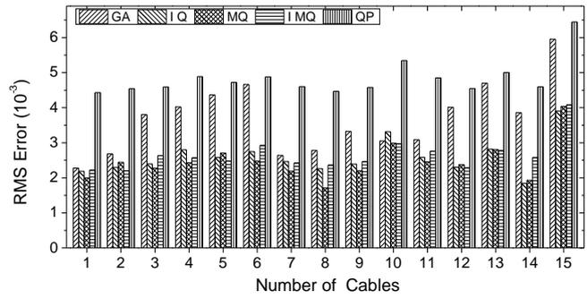
(b) The RMS error of cable tensions
